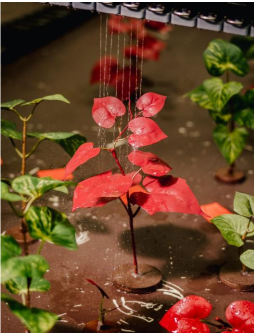
A Blue River prototype sprays water on the red plants.
